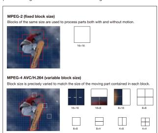
accuracy of motion compensation to boost the quality of fast-motion images while increasing compression efficiency.
